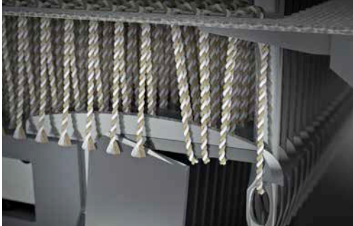
Pick-up of the loop by the looper
